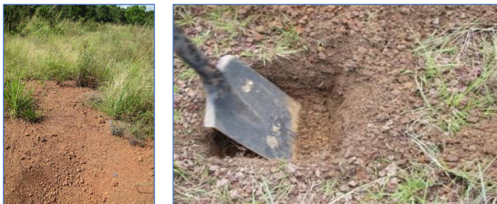
Image 1. Soils of the project area. The continuous burning of grasses on soils with oxisol characteristics causes a hard layer of ferrous material called plinthite to form 15 .
